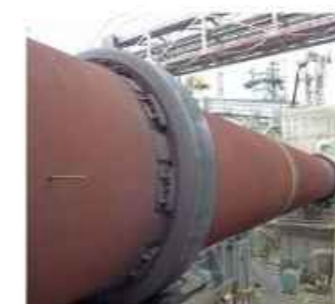
Rotary kiln for calcining dehydrated cakes
